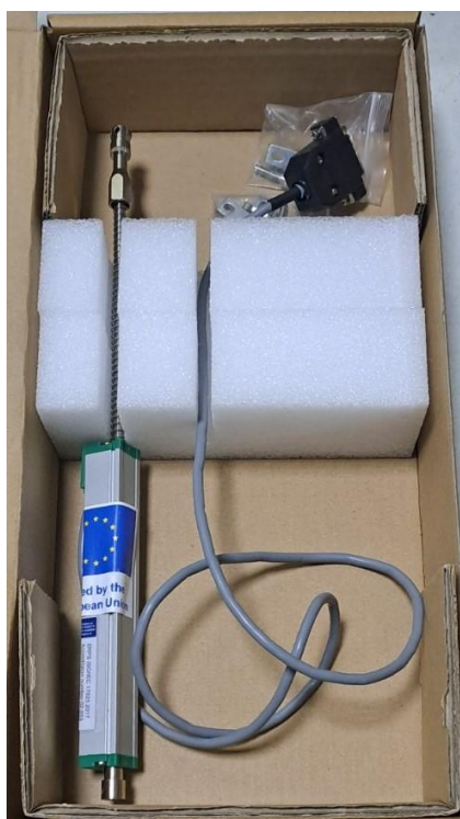
Linear potentiometer with active range 100mm
